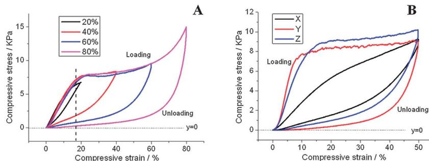
**Fig. 2** (A) Loading and unloading compressive stress–strain curves of several ECFs at different set strains of 20%, 40%, 60%, and 80%, respectively. (B) Stress–strain curves recorded by compressing a cubic ECF along three orthogonal directions at compression strains of 50% (X: length, Y: width, Z: thickness).
