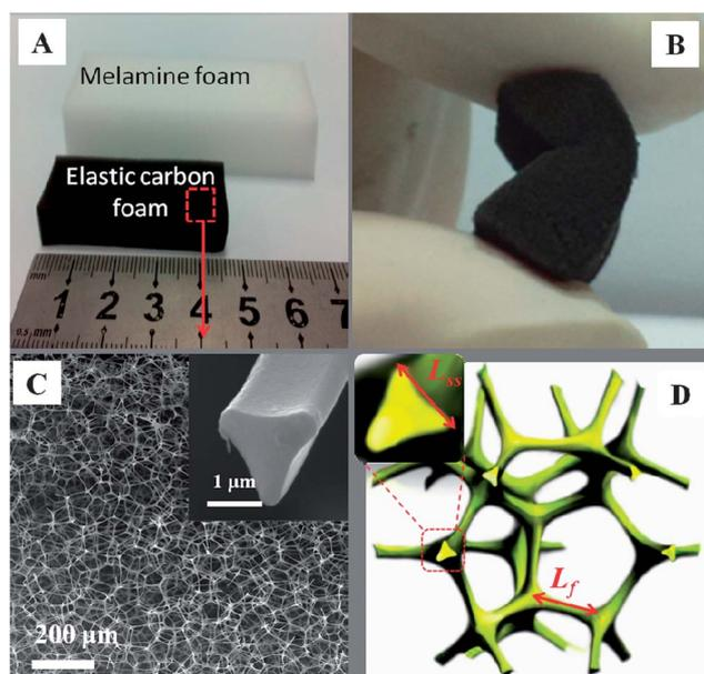
**Fig. 1** Digital photos of (A) a piece of MF with a size of 70 × 18 × 20 mm and the derived ECF with a size of 46 × 10 × 13 mm and (B) ECF bent by finger tips. (C) Scanning electron microscopy image of ECF, inset is the cross-sectional image of one network fiber in the ECF, which shows a concave regular triangle shape. (D) Model for the ECF architecture.
