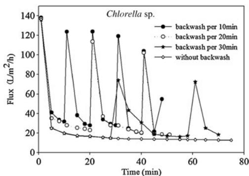
Fig. 3 Flux with different backwash frequency
