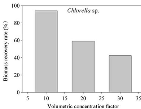
Fig. 5 Effect of volume concentration factor on biomass recovery
