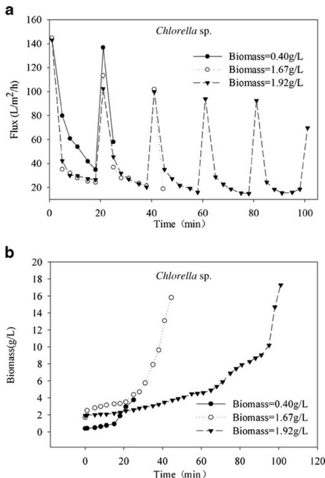
Fig. 4 Flux and biomass with different initial biomass. a Flux with different initial biomass. b Recovered biomass with different initial biomass density
