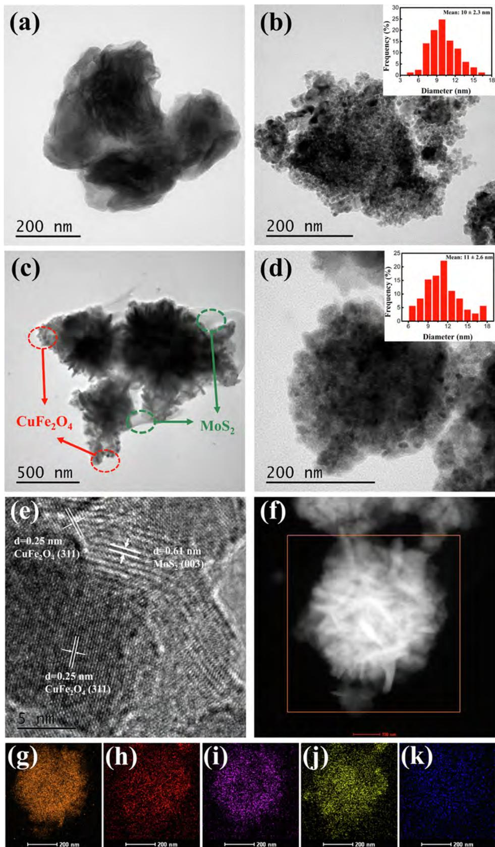
**Fig. 2.** Transmission electron microscope pictures of (a) MoS<sub>2</sub>, (b) CuFe<sub>2</sub>O<sub>4</sub>, and (c-d) MC1.5; (e) high-resolution transmission electron microscope; (f) high angle annular dark-field scanning transmission electron microscope images and corresponding element mapping images of MC1.5 for (g) S, (h) Mo, (i) O, (j) Fe, and (k) Cu. The inset of (b) and (d) is the corresponding particle size distribution of nano-CuFe<sub>2</sub>O<sub>4</sub>.
