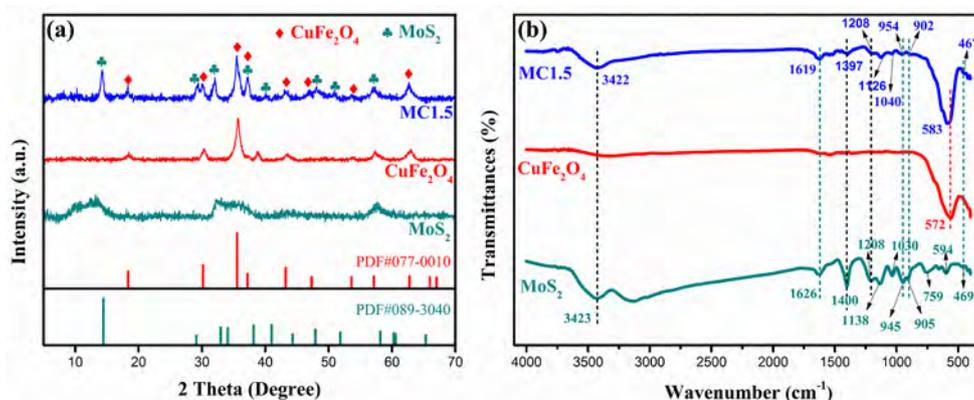
Fig. 1. (a) X-ray diffraction patterns and (b) fourier transform infrared spectra of as-prepared catalysts.
