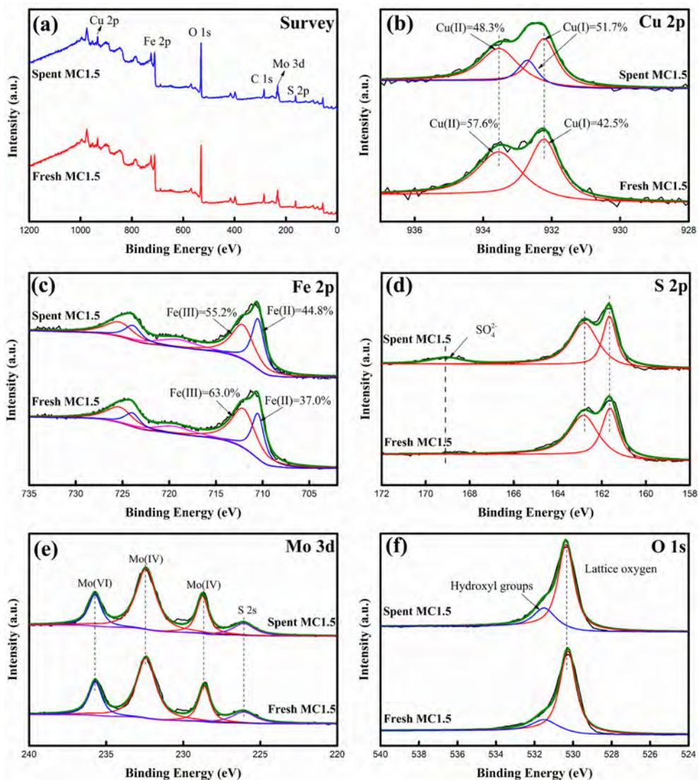
Fig. 4. (a) X-ray photoelectron spectroscopy (XPS) survey, (b) Cu 2p XPS spectra, (c) Fe 2p XPS spectra, (d) S 2p XPS spectra, (e) Mo 3d XPS spectra, and (f) O 1s XPS spectra of  $\text{MoS}_2/\text{CuFe}_2\text{O}_4$  before and after the reaction.
