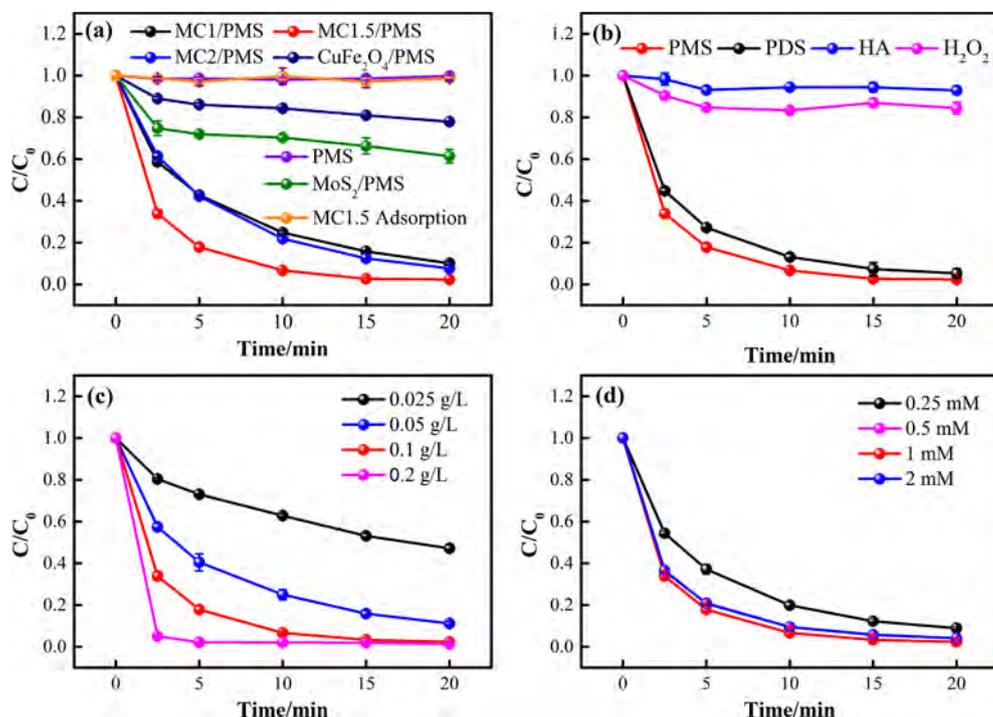
Fig. 3. (a) The degradation efficiency of fluoxetine under various material ratios; the effects of (b) different system, (c) different catalyst dosages, and (d) peroxymonosulfate concentration on the degradation of fluoxetine. Experimental conditions: catalysts = 0.1 g/L, oxidant = 1 mM, initial pH = 6.9, stirring speed = 300 rpm, and T = 25 °C. PMS: peroxymonosulfate; PDS: persulfate; HA: hydroxylamine hydrochloride; H<sub>2</sub>O<sub>2</sub>: hydrogen peroxide.
