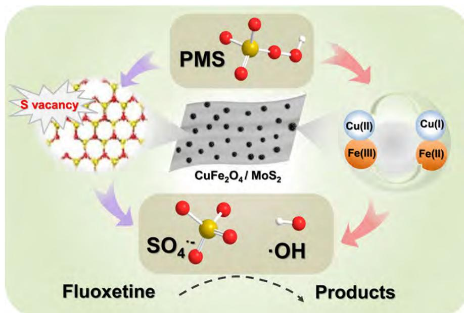
Fig. 6. Proposed generation mechanism of radicals in the MoS<sub>2</sub>/CuFe<sub>2</sub>O<sub>4</sub>/peroxymonosulfate system.
