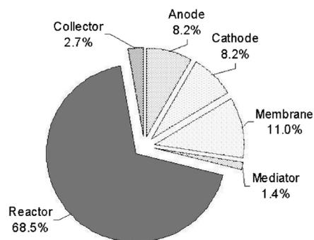
**Figure 3.** Comparison of the estimated costs of laboratory systems. The following cost assumptions were used: the reactor is constructed from oroglas materials, and operational costs are approximately 250 USD for a 1 m<sup>3</sup> cubic MFC, the anode and cathode (1 m<sup>2</sup>, graphite felt) each cost 30 USD, the ion-exchange membrane (1 m<sup>2</sup>) costs 40 USD, the collector (titanium wire) costs 10 USD; and the nanocatalyst or mediator (phthalocyanine or ferricyanide) cost 5 USD.
