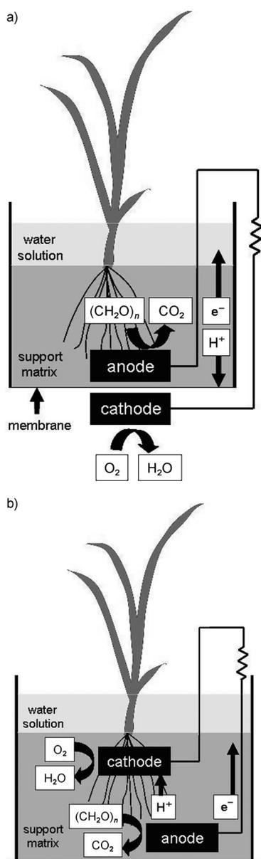
**Figure 2.** Modified configurations of PMFCs. a) A configuration with a membrane fixed at the bottom with one side in contact with the sediment, in which the anode is located, and the cathode is located on the other side of the membrane. b) Oxygen released from the root can be used as the electron acceptor at the cathode in a single-chamber PMFC.<sup>[27]</sup>
